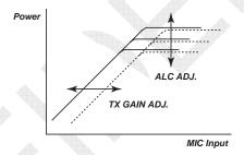
Fig. 7.2.6 Correlation between ALC and TX Gain Adjustment
