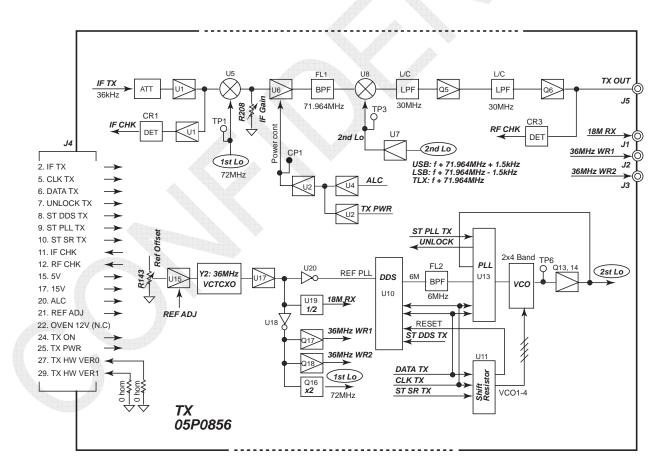
Fig. 7.2.1 TX Board Block Diagram
