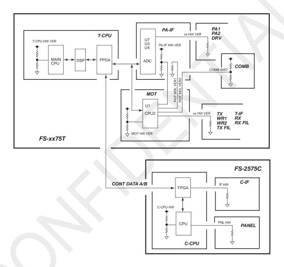
Fig. 6.5.1 Version Verification Circuit Diagram for FS-5075
