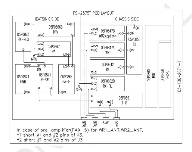
Fig. 2.3.5 FS-2575T, PCB LAYOUT
