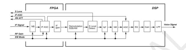
Fig. 7.6.4 Overview of Configuration of Reception/Demodulation Processing Line
