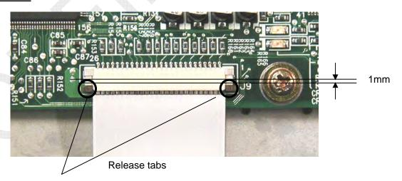
Note 2) Disconnecting flat cable from FDD connector
