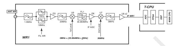
Fig. 6.1.2 WR1 Test Circuit Diagram
