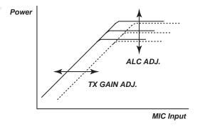
Fig. 5.7.18 Relationship between ALC and TX GAIN
