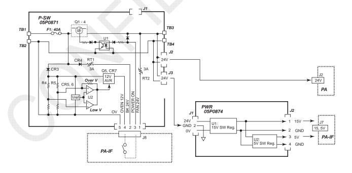
Fig. 7.7.3 FS-1575 Power Supply Circuit Block Diagram
