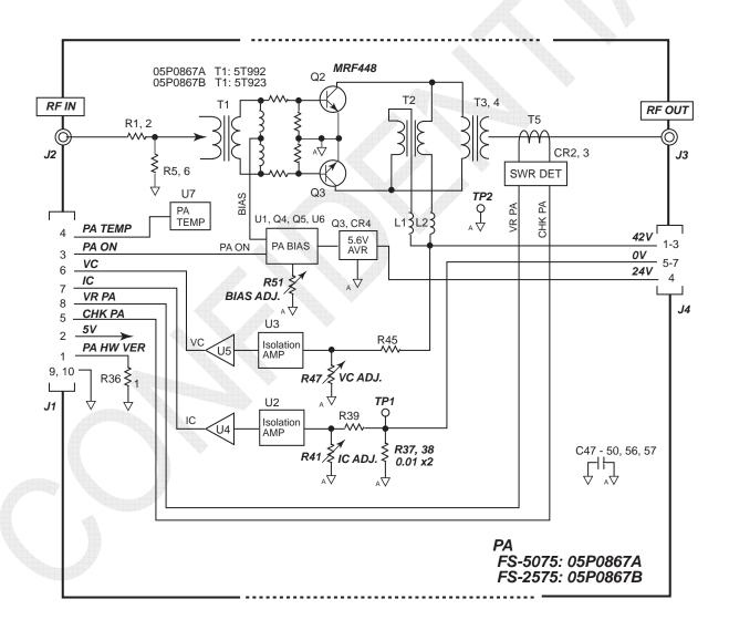
Fig. 7.2.9 FS-2575/FS-5075 PA Board Block Diagram
