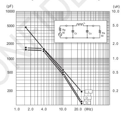
Fig. 7.9.9 Pi-matching Measurement Constant for 50-ohm Loads
