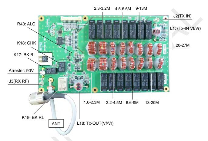
Fig. 2.5.1 TX-FIL board (05P0876) A-side
