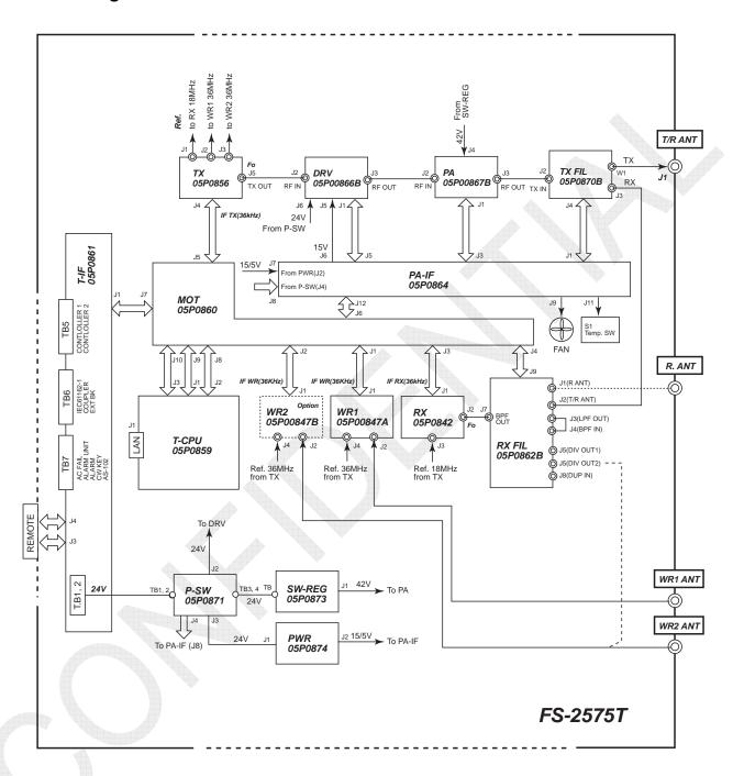
Fig. 7.1.3 Configuration of FS-2575T Transceiver Unit
