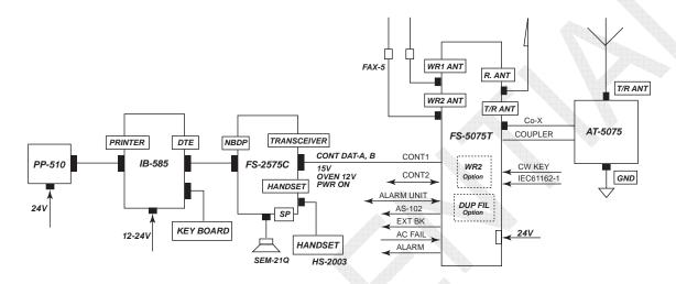
Fig. 7.1.1 FS-5075 System Configuration
