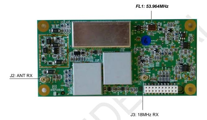
Fig. 2.5.31 RX board (05P0842) A-side
