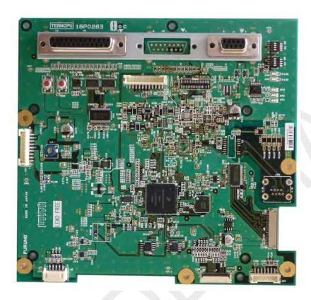
Fig. 2.7.16 TERM CPU board (16P0283A)A-side
