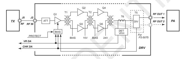
Fig. 6.1.10 DRV CHK Circuit Diagram
