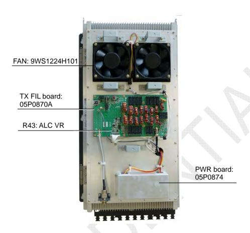
Fig. 2.4.3 FS-5075T, front cover removed
