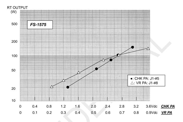
Fig. 6.11.10 FS-1575 PA Board - Example of CHK PA, VR PA vs. Power Characteristics
