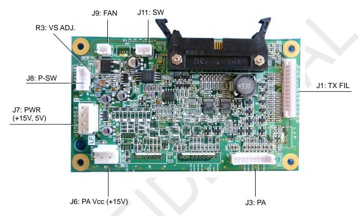
Fig. 2.5.23 PA-IF board (05P0864A) A-side
