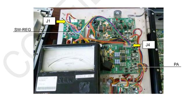
Fig. 5.7.5 FS-2575: Example of Ammeter Connection
