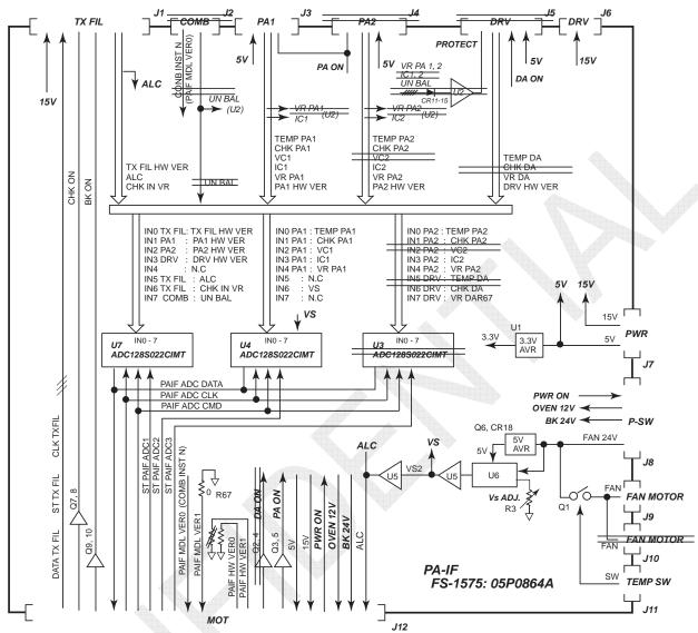
Fig. 7.2.16 PA-IF Board (05P0864A) Block Diagram
