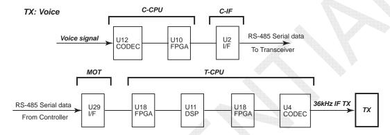
Fig. 7.6.6 Overview Diagram of Transmitted Voice Signal Channel
