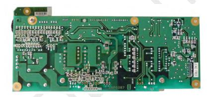
Fig. 2.7.19 TERM PWR board (16P0287A) B-side
