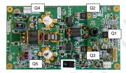
Example: FS-2575 @4M, +5dBm input, Output; 10W
