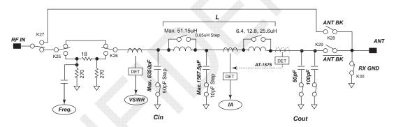
Fig. 7.9.3 Matching Circuit Block Diagram
