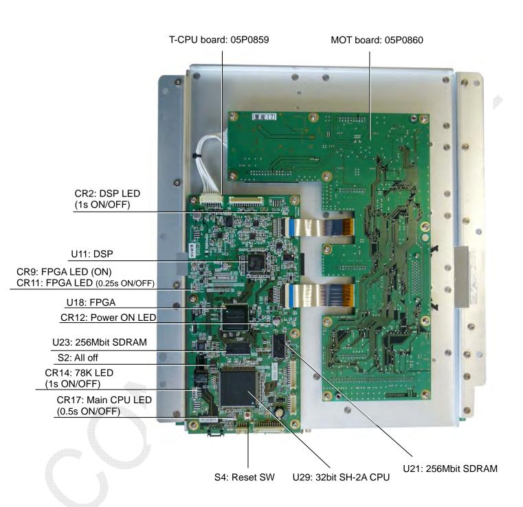
Fig. 2.2.8 FS-1575T, mounting board (B-side)
