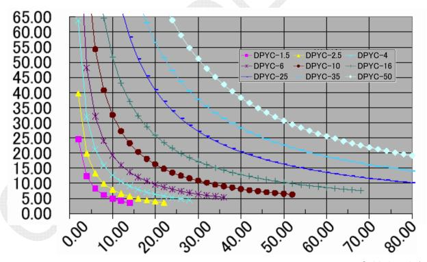
Fig. 1.2.2 Voltage Drops in Cables:5%
