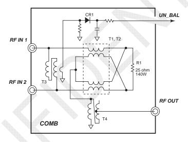
Fig. 7.2.13 COMB Board Block Diagram
