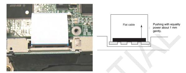
Note 2) Disconnecting flat cable from FDD connector To disconnect the flat cable;
