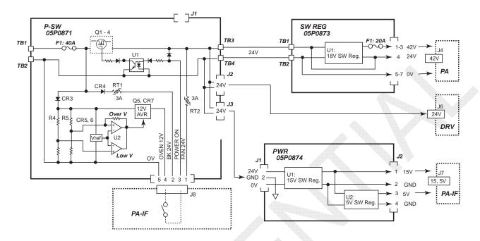
Fig. 7.7.2 FS-2575 Power Supply Circuit Block Diagram
