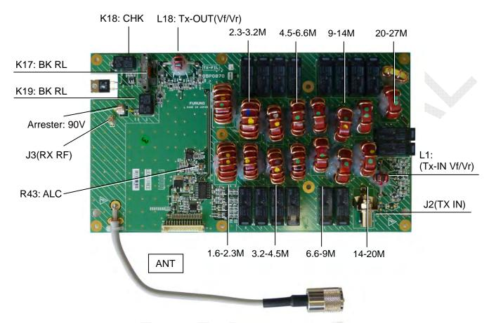
Fig. 2.5.5 TX-FIL board (05P0870A) A-side
