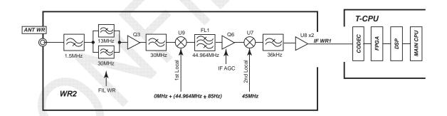
Fig. 6.1.3 WR2 Test Circuit Diagram
