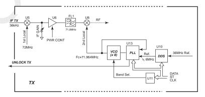
Fig. 6.1.8 TX PLL CHK Circuit Diagram
