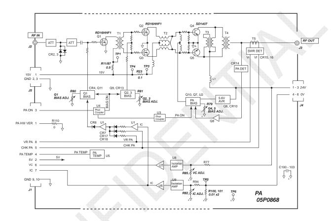
Fig. 7.2.12 FS-1575 PA Board Block Diagram
