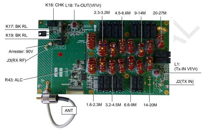
Fig. 2.5.3 TX-FIL board (05P0870B) A-side
