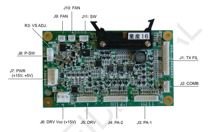
Fig. 2.5.21 PA-IF board (05P0864) A-side
