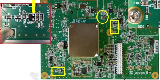
J1: 18MHz RX 200mVp-p (when terminated through a 50-ohm resistor)
