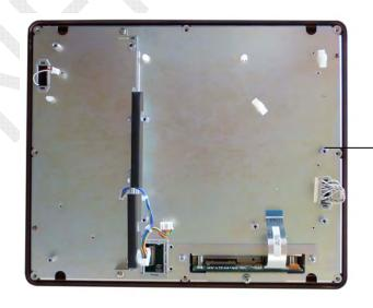
Mounting chassis of LCD panel
