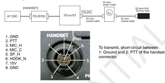
Fig. 5.7.23 ALC Adjustment Circuit
