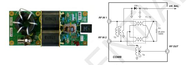
Fig. 6.11.12 FS-5075 - COMB Board Block Diagram
