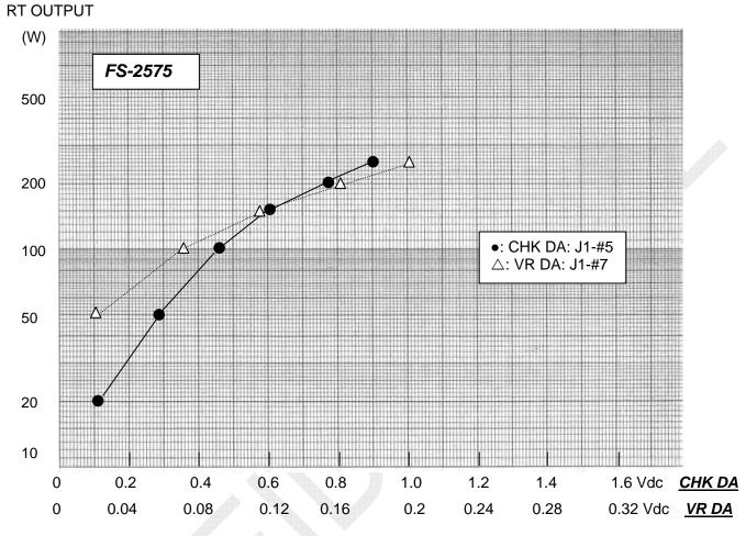
Fig. 6.11.3 FS-2575 DRV Board - Example of CHK DA, VR DA vs. Power Characteristics
