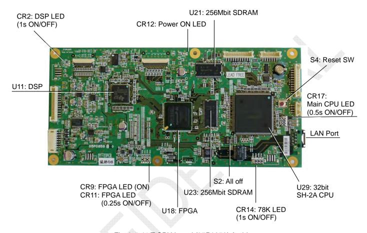
Fig. 2.5.41 T-CPU board (05P0859) A-side
