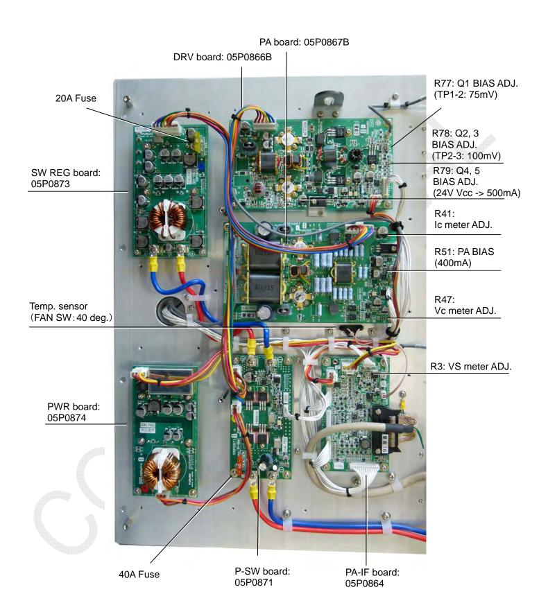
Fig. 2.3.7 FS-2575T, heat sink side
