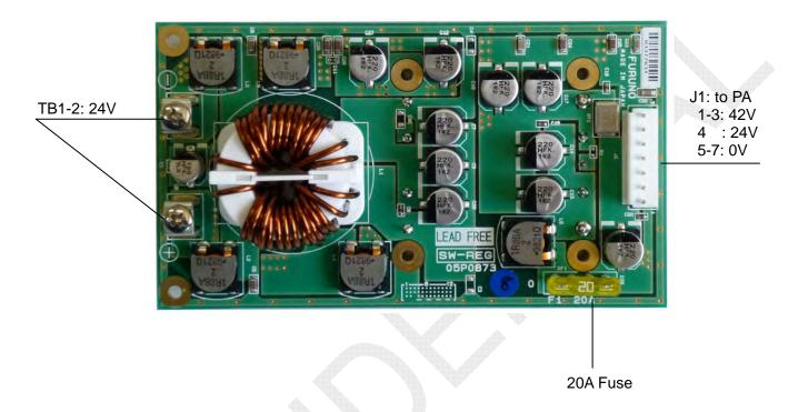
Fig. 2.5.43 SW-REG board (05P0873) A-side
