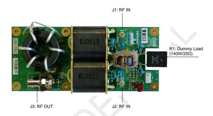
Fig. 2.5.7 COMB board (05P0869) A-side
