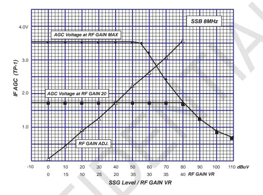
Fig. 7.3.8 Example of IF AGC Characteristics
