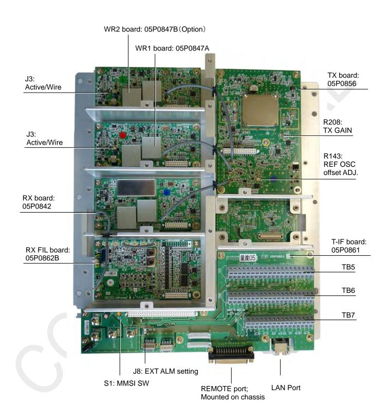
Fig. 2.3.8 FS-2575T, mounting board (A-side)
