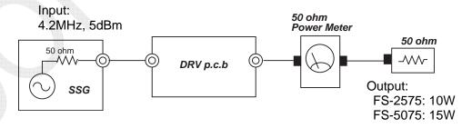
Fig. 6.11.4 Power Check Using DRV Board Alone
