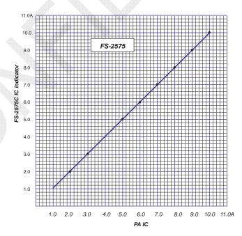
Fig. 5.7.8 FS-2575: Example of PA IC Reading Characteristics
