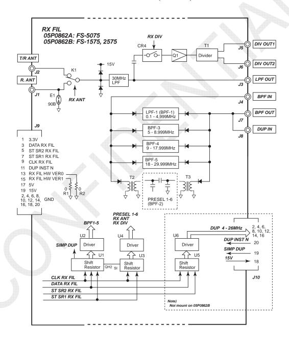
Fig. 7.3.1 RX FIL Board Block Diagram
