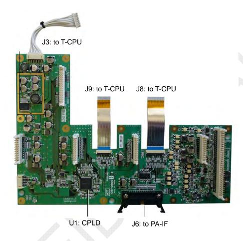
Fig. 2.5.39 MOT board (05P0860) A-side
