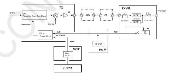
Fig. 5.7.24 ALC Control Circuit Diagram
