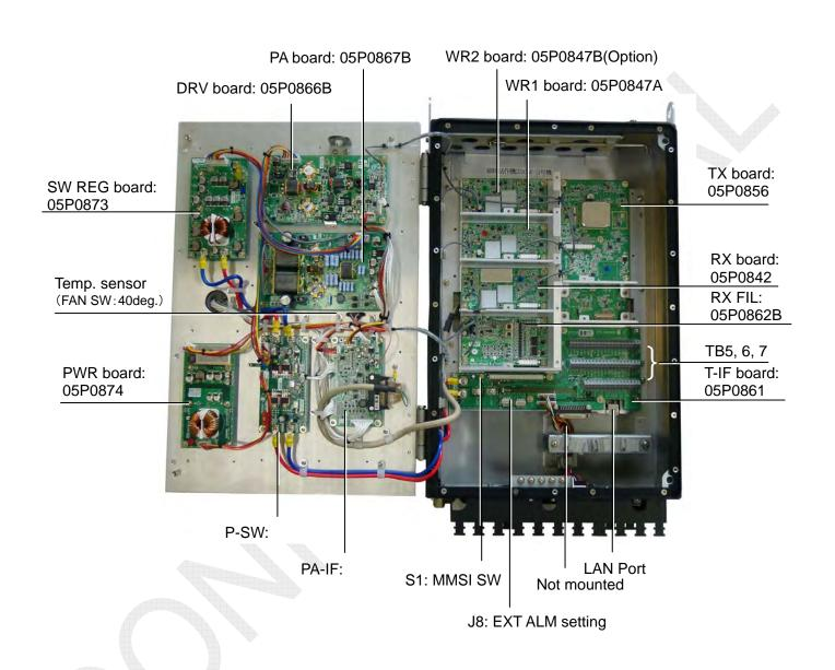
Fig. 2.3.6 FS-2575T, shield cover removed
