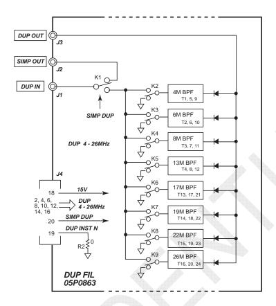
Fig. 7.3.5 DUP FIL Board Block Diagram
