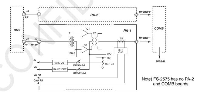
Fig. 6.11.5 FS-2575 and -5075 - PA Board Block Diagram
