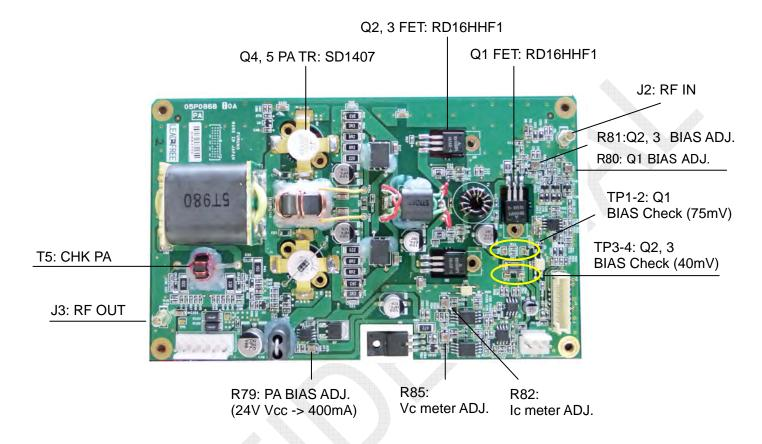
Fig. 2.5.9 PA board (05P0868) A-side
