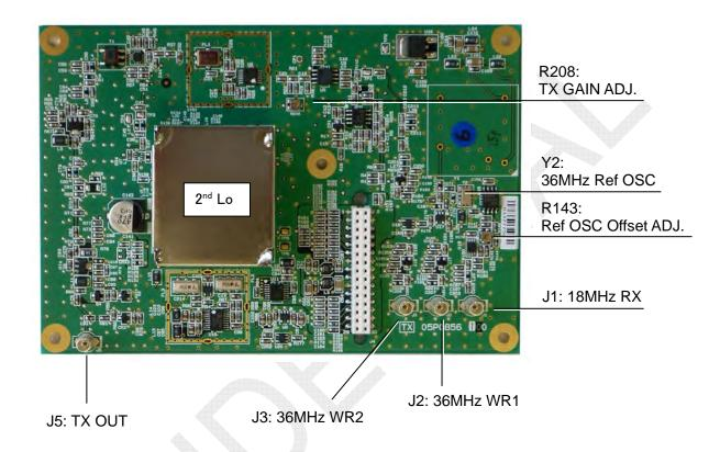
Fig. 2.5.19 TX board (05P0856) A-side
