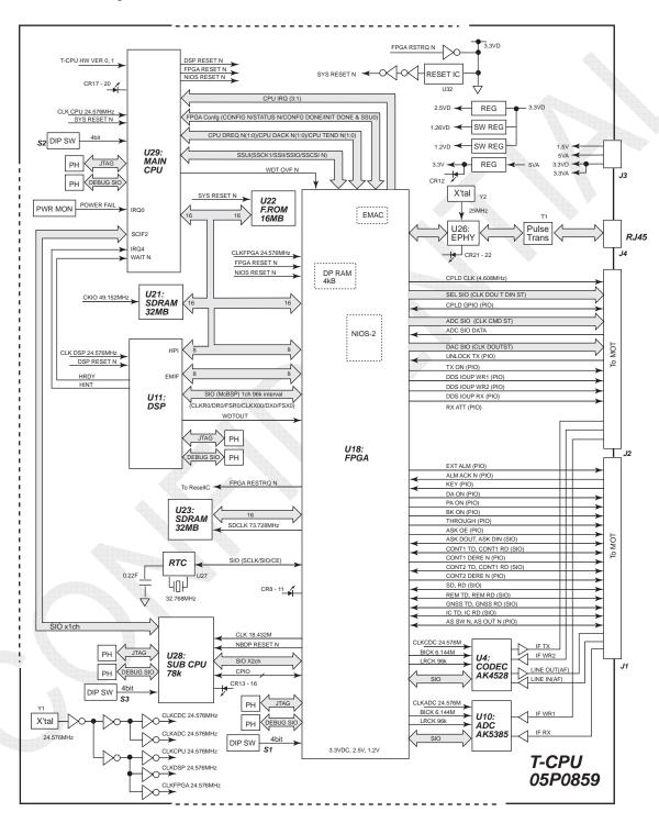
Fig. 7.6.1 T-CPU Board (05P0859) Block Diagram
