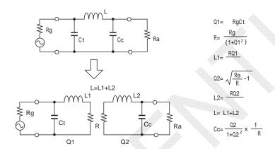
Fig. 7.9.8 Calculation of Pi-matching
