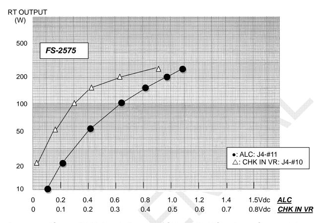
Fig. 6.11.15 FS-2575 TX FIL Board - Example of CHK IN VR, ALC vs. Power Characteristics
