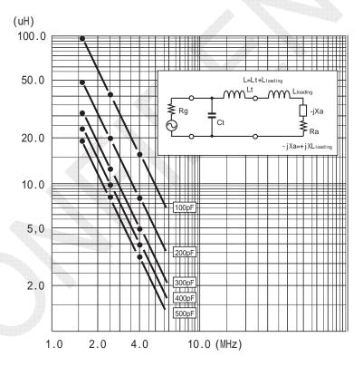
Fig. 7.9.7 Table of Loading Coil Constants
