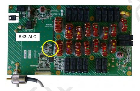
Fig. 5.7.21 TX FIL Board (05P0870A, B): FS-2575 and FS-5075
