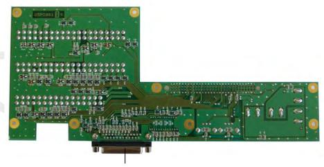
[REMOTE] mounted: 05P0861A (For FS-1575) [REMOTE] not mounted: 05P0861
