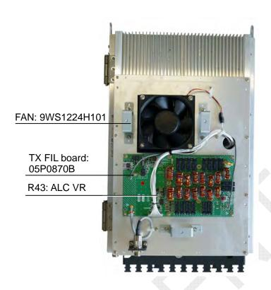
Fig. 2.3.3 FS-2575T, front cover removed
