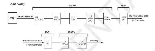
Fig. 7.6.12 Overview Diagram of WR2 Signal Channel
