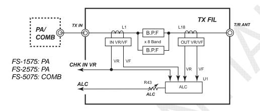
Fig. 6.11.13 TX FIL Board Block Diagram
