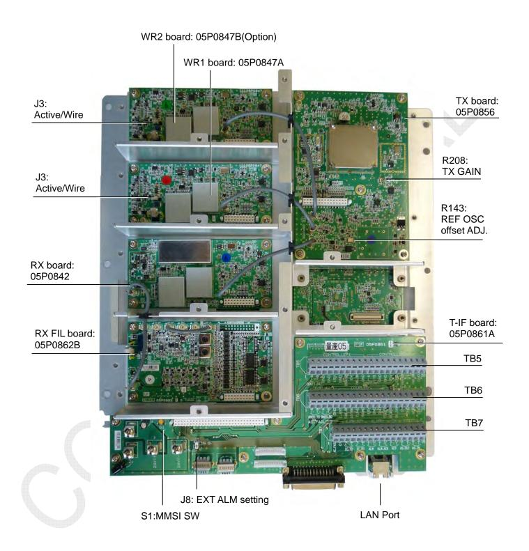
Fig. 2.2.7 FS-1575T, mounting board (A-side)
