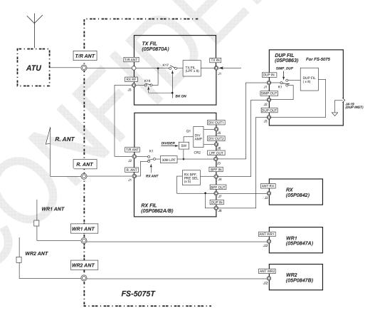
Fig. 7.3.4 Example of Installation Pattern for Duplex Specification
