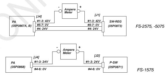
Fig. 5.7.7 PA IC Reading Adjustment Circuit
