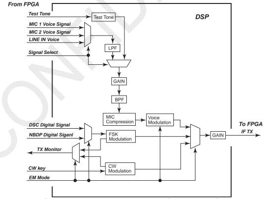
Fig. 7.6.3 Overview of Transmission Processing Circuit within DSP Transmitter
