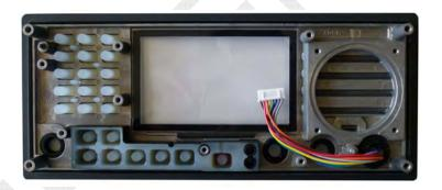
Fig. 2.1.7 Front panel, PANEL board removed
