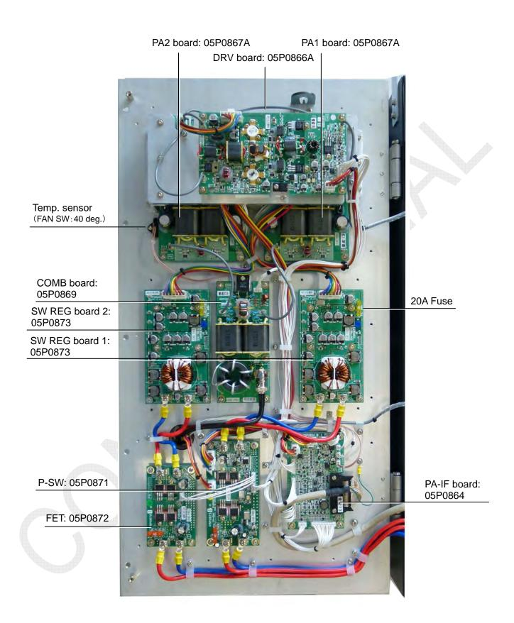
Fig. 2.4.7 FS-5075T, heat sink side
