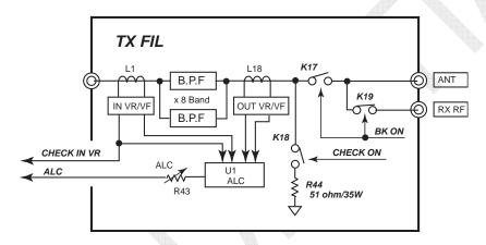
Fig. 6.1.13 TX FIL CHK Circuit Diagram
