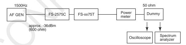
Fig. 5.1.2 1-Tone Measurement Circuit
