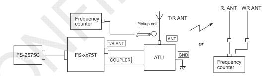
Fig. 5.4.1 Frequency Measurement Circuit
