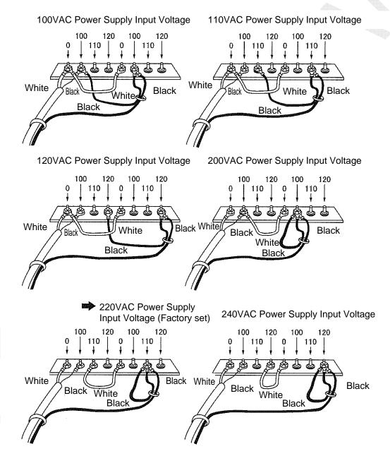
Fig. 4.16.1 PR-850A Input Power Supply Voltage
