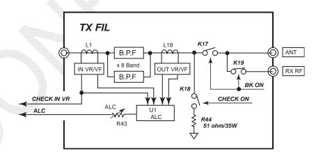
Fig. 6.1.5 TX FIL board CHK signal
