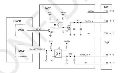
Fig. 1.2.3 FS-xx75 Block Circuit Diagram
