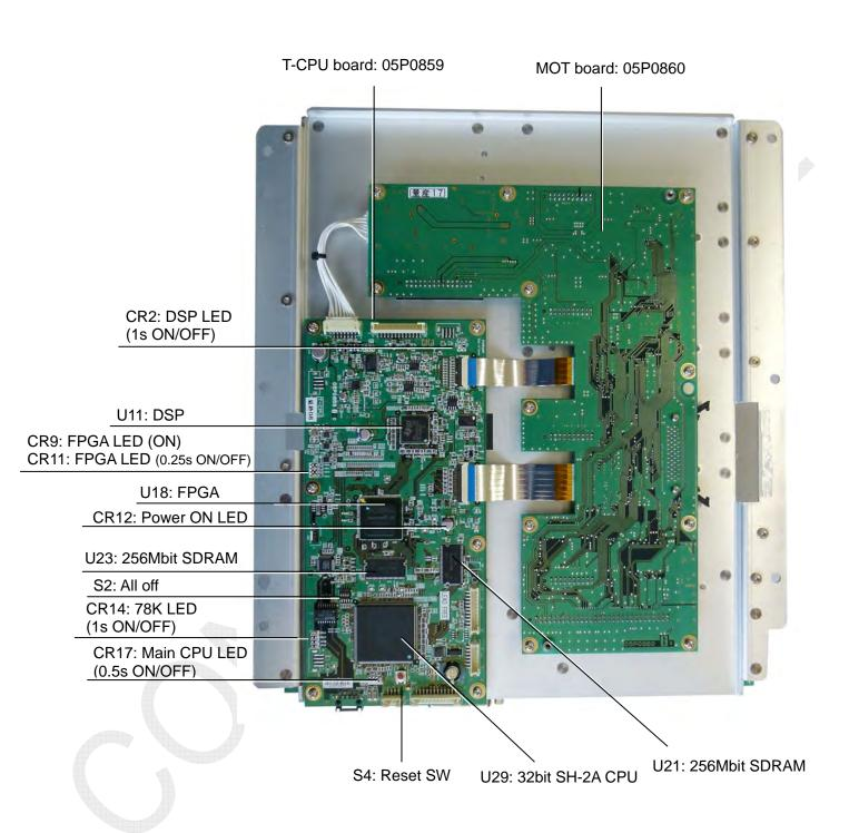
Fig. 2.3.9 FS-2575T, mounting board (B-side)
