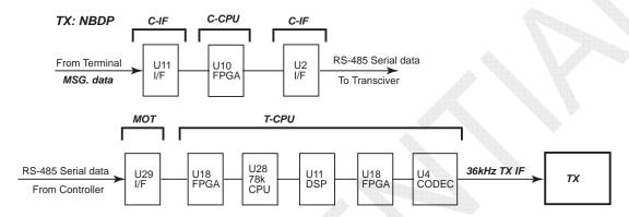
Fig. 7.6.8 Overview Diagram of Transmitted NBDP Signal Channel
