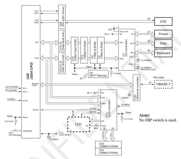
Fig. 7.10.4 TERMCPU Board Block Diagram
