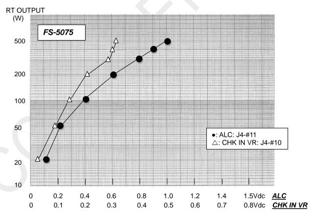
Fig. 6.11.14 FS-5075 TX FIL Board - Example of CHK IN VR, ALC vs. Power Characteristics
