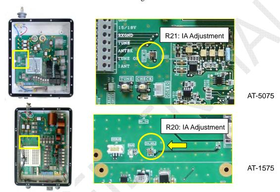
Fig. 5.7.26 Location of ATU IA ADJ. Variable Resistors
