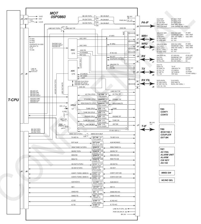
Fig. 7.5.2 MOT Board Block Diagram
