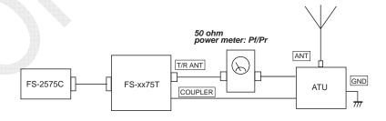
Fig. 5.3.2 Output Power Measurement circuit-2
