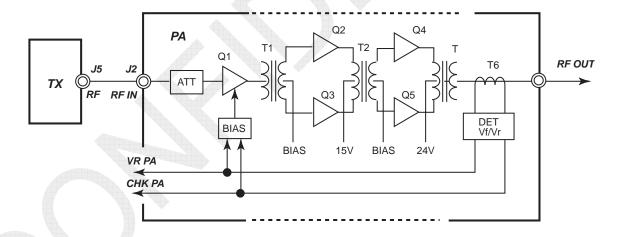
Fig. 6.11.9 FS-1575 - PA Board Block Diagram
