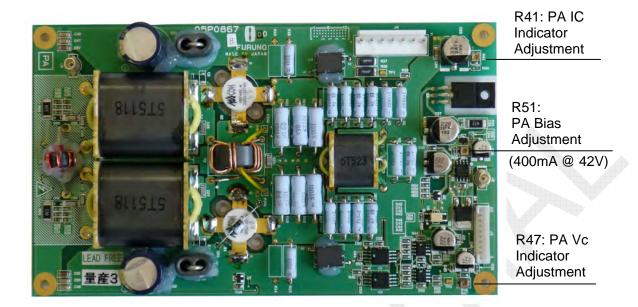
Fig. 5.7.2 FS-5075, FS-2575 PA Board (05P0867A, B)
