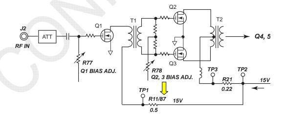
Fig. 5.7.15 DRV Board: Q1 BIAS Circuit
