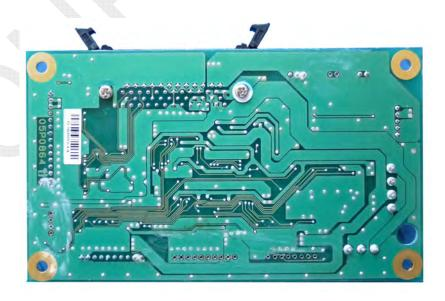
Fig. 2.5.24 PA-IF board (05P0864A) B-side
