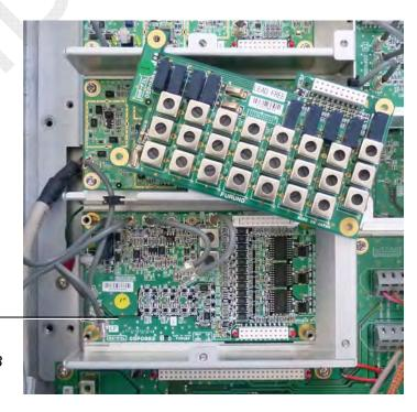
Fig. 2.4.10 FS-5075T, RX-FIL and DUP FIL board
