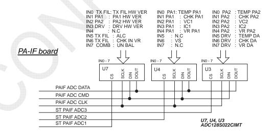
Fig. 6.1.6 Signals Detected by TX SELF TEST
