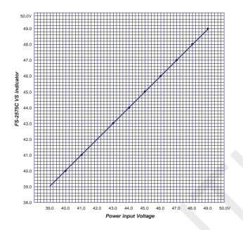
Fig. 5.7.6 FS-2575: Example of Vc Reading Characteristics
