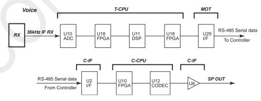
Fig. 7.6.7 Overview Diagram of Received Voice Signal Channel
