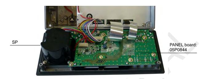
Fig. 2.1.6 Front panel opened
