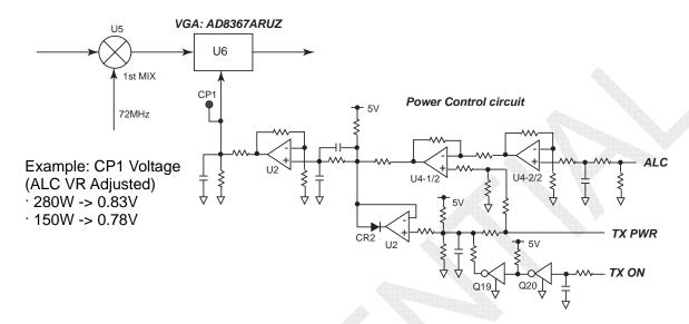
Fig. 7.2.4 TX Board Power Control Circuit
