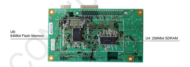
Fig. 2.1.10 C-CPU board: 05P0852 (B-side)
