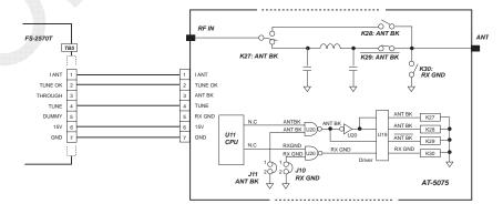
Fig. 4.12.3 Connection between FS-2570 and AT-5075
