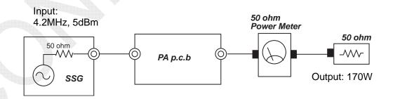
Fig. 6.11.11 FS-1575 - Power Check Using PA Board Alone
