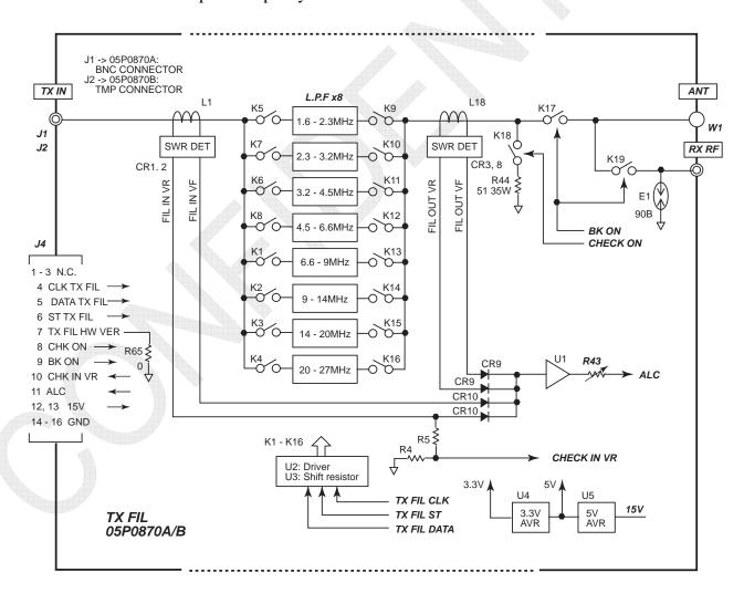
Fig. 7.2.14 TX FIL Board Block Diagram
