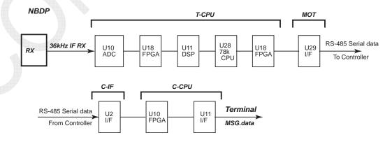
Fig. 7.6.9 Overview Diagram of NBDP RX IF Signal Channel
