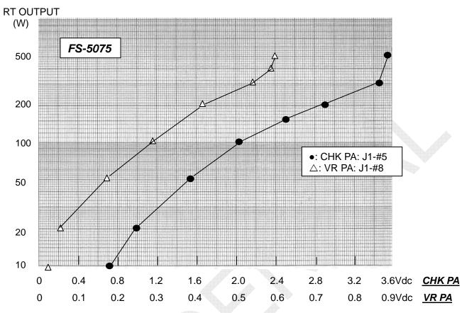
Fig. 6.11.6 FS-5075 PA Board - Example of CHK PA, VR PA vs. Power Characteristics
