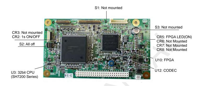
Fig. 2.1.9 C-CPU board: 05P0852 (A-side)
