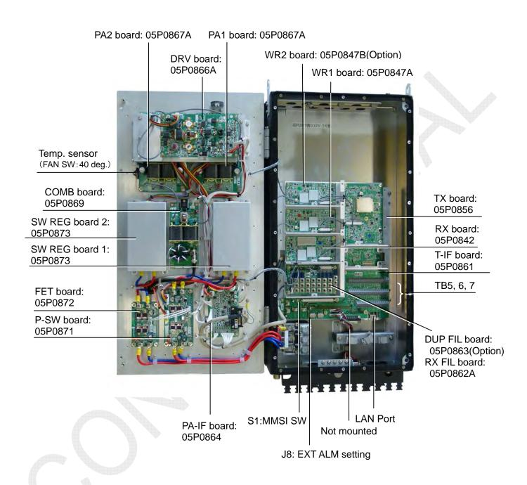
Fig. 2.4.6 FS-5075T, shield cover removed
