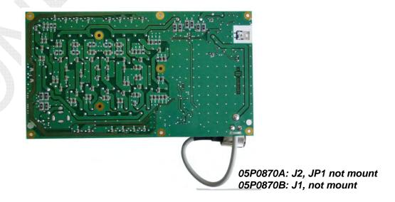
Fig. 2.5.4 TX-FIL board (05P0870B) B-side
