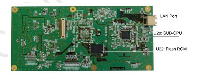
Fig. 2.5.42 T-CPU board (05P0859) B-side
