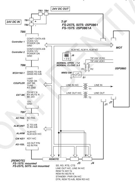
Fig. 7.5.1 T-IF Board Block Diagram
