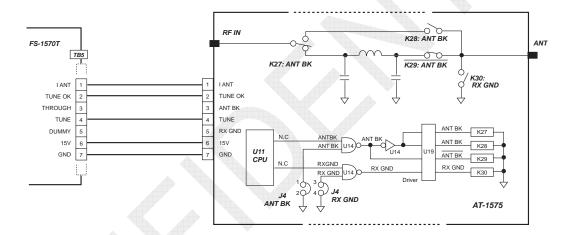
Fig. 4.13.2 Connection between FS-1570 and AT-1575
