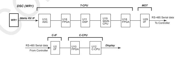
Fig. 7.6.11 Overview Diagram of WR1 IF Signal Channel
