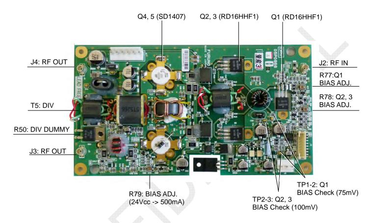
Fig. 2.5.17 DRV board (05P0866A) A-side
