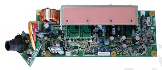
Fig. 2.7.18 TERM PWR board (16P0287A) A-side
