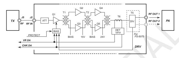
Fig. 6.11.1 DRV Board Block Diagram
