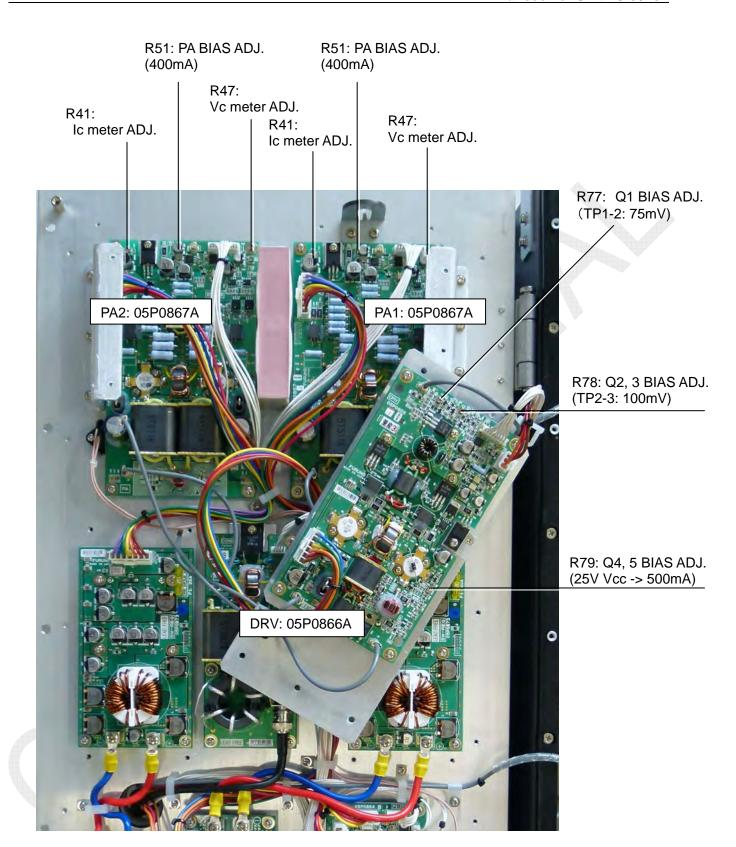
Fig. 2.4.8 FS-5075T, DRV board removed
