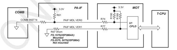
Fig. 6.5.3 INST Signal of COMB / PA-IF Board
