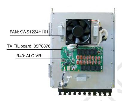
Fig. 2.2.3 FS-1575T, front cover removed
