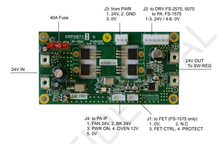
Fig. 2.5.47 P-SW board (05P0871) A-side
