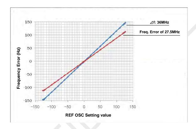
Fig. 5.4.2 Example of REF OSC Characteristics
