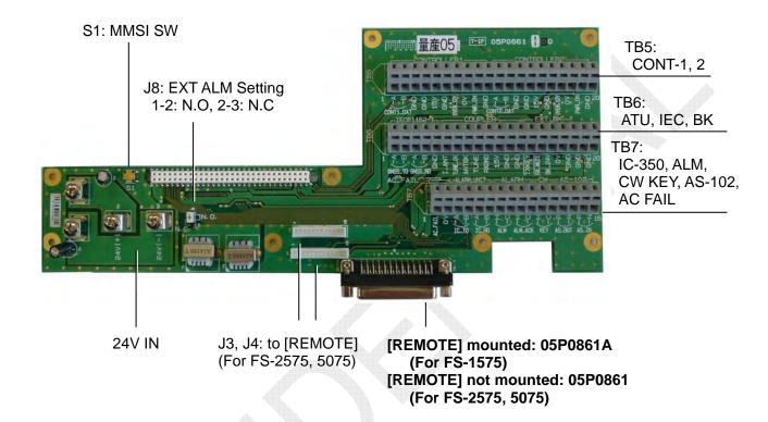
Fig.5.37 T-IF board (05P0861A) A-side
