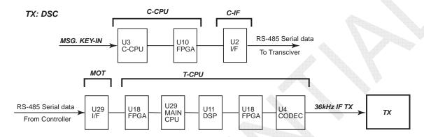
Fig. 7.6.10 Overview Diagram of Transmitted DSC Signal Channel
