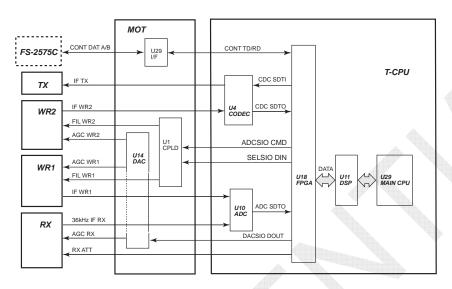
Fig. 7.6.2 Overview of 36-kHz IF Signal Channels
