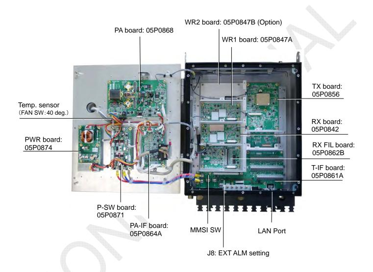
Fig. 2.2.5 FS-1575T, shield cover removed
