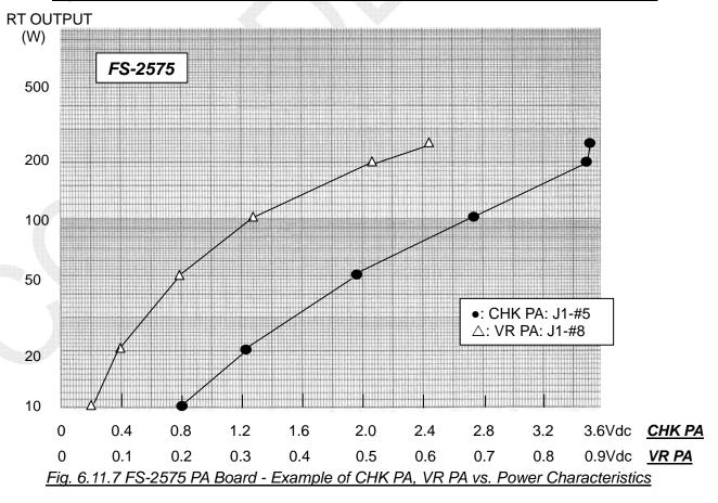
To check for output power using the DRV board plus the PA board alone, the SSG signal can be used as an input signal. Output values are just for reference.
