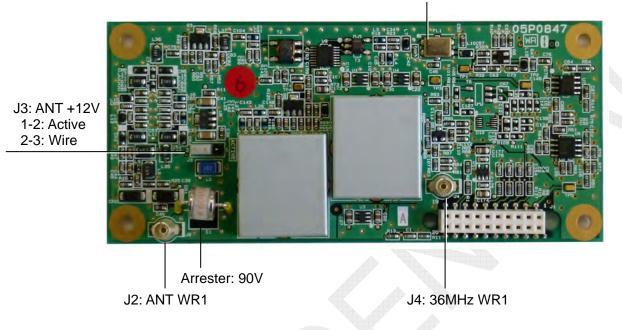
Fig. 2.5.33 WR1 board (05P0847A) A-side
