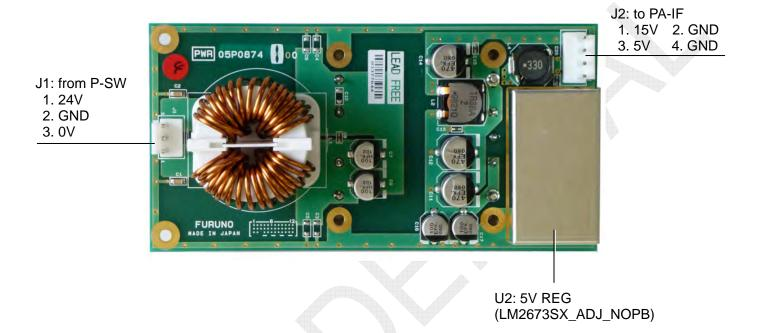
Fig. 2.5.45 PWR board (05P0874) A-side
