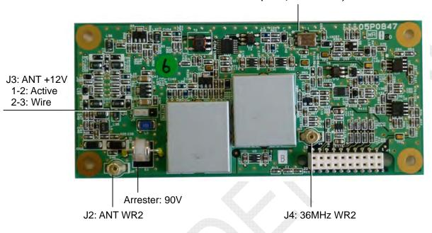
Fig. 2.5.35 WR2 board (05P0847B) A-side
