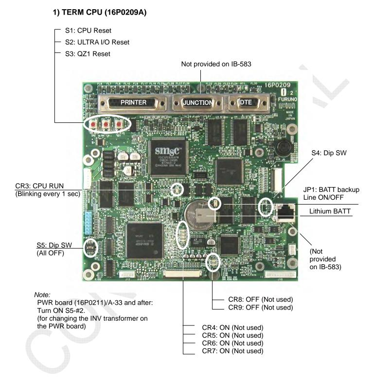
Fig. 2.7.7 TERM CPU board (16P0209A)
